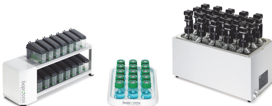
Figure 2 The Gas Endeavour with 500 ml bottles and mechanical agitation in a thermostatic water bath.
